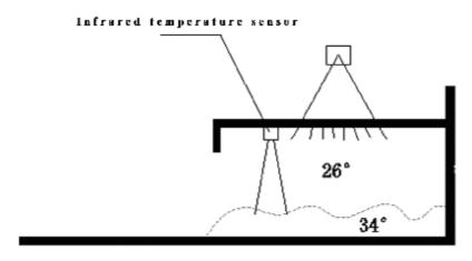
Open a hole on the top cover, then slotting the infrared temperature sensor into the round hole, using provided self tapping screws to fasten the sensor on the top cover of the box. As shown in the following figure:
