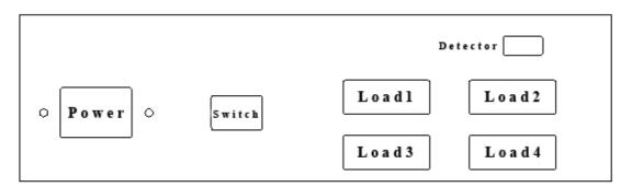
Power: 220VAC InputSwitch: Turn on/off powerLoad1: Heat lamp or heat mat inputLoad2: Heat lamp or heat mat inputLoad3: Heat lamp or heat mat inputLoad4: Heat lamp or heat mat inputDetector: Infrared thermal sensor input
