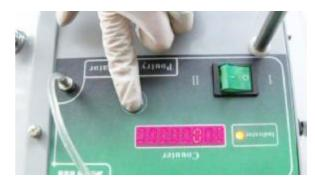
4) Press the Reset Button to zero the counter on the LED screen.
